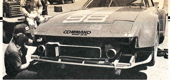
With front air dam removed, front wing of Walt Bohren car is visible. Airflow over wing creates front downforce, increasing steering effort by as much as 50%, according to Kent. Kent balances front downforce by increasing rear spoiler height. Mueller prefers a more conventional setup, with very neutral handling.
