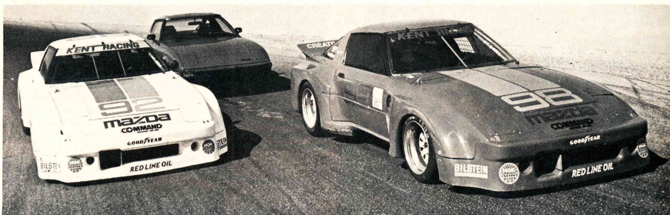
On-track shot shows visual differences between race-prepped RX-7s and box stocker. Racers' engine air enters through square opening, radiator air through narrower horizontal slot. Round holes pipe air directly onto front brake rotors.
