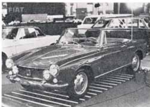
Latest version of the 1600S Fiat has a scooped bonnet and four headlights. The twin o.h.c. 1.6-litre engine develops 100 b.h.p. Another model, the 1500 Cabriolet has the same body/structure with 1½-litre pushrod "saloon" engine, two headlights, and a 100 m.p.h. maximum.
